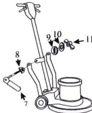
When correctly installed, the collar slides easily when the cam-engineered locking lever is "up", but is firmly fixed when the lever is "down".
