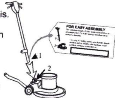
1. Remove the handle and mounting hardware from the carton. Bolts, nuts, washers, and the locking lever assembly are in the plastic bag attached to the handle.
